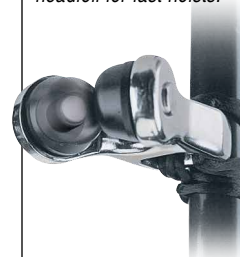
Prefeeder: Hardcoat-anodized, PTFE-coated aluminum rollers spin freely on low-friction bushings.
