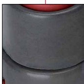
6061-T6 aluminum: Hard Lube-anodized
